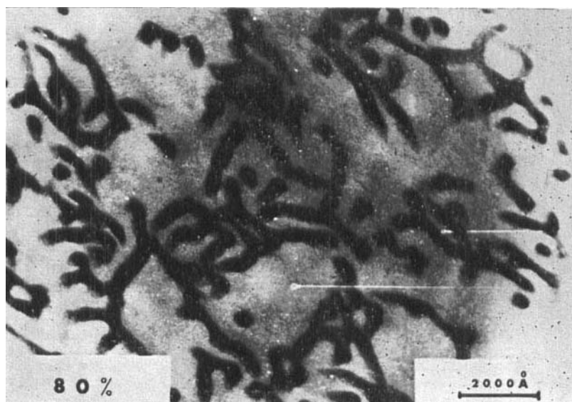
Figure 11. Electron micrograph of the copolymer SB. 1 plus 80% polystyrene.
