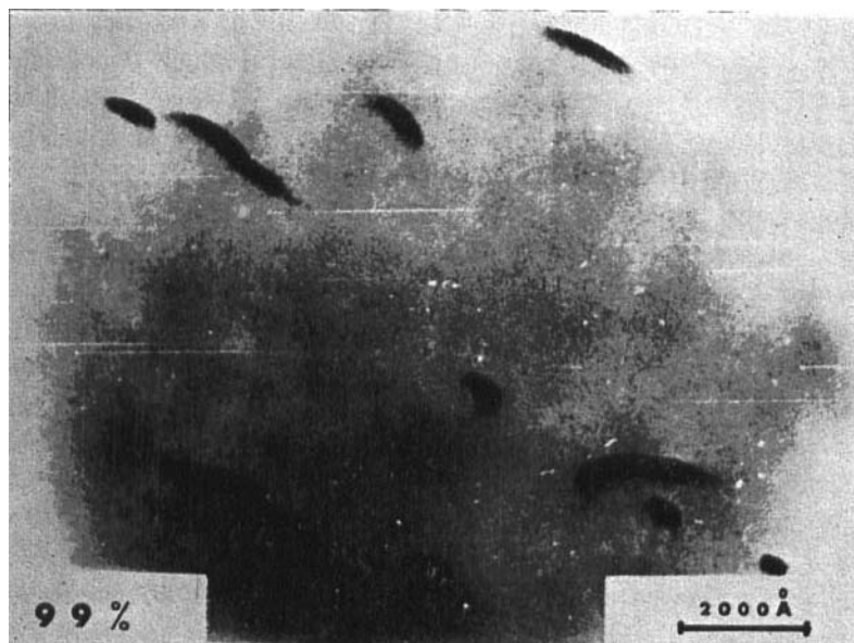
Figure 14. Electron micrograph of the copolymer SB. 1 plus 99% polystyrene.
